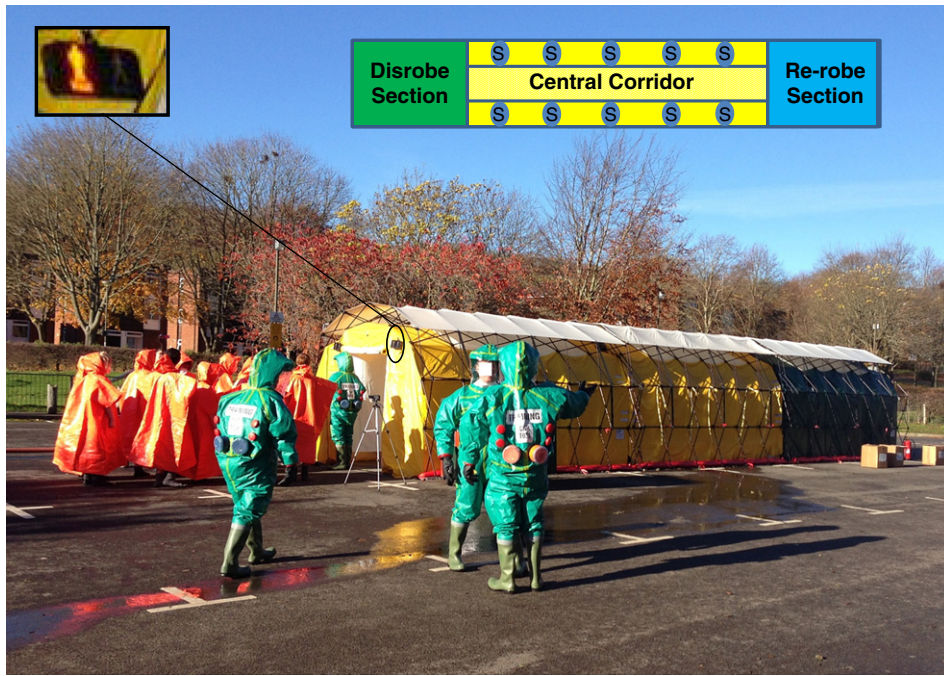
Fig. 7. Mass casualty decontamination unit (“MD1”) deployed by UK specialist responders. Photograph acquired during an exercise and shows a group of 10 individuals in high visibility ponchos (Fig. 5) waiting to enter disrobe area in accordance with a “traffic light” system (inset, top left). Schematic of unit (inset, top right) indicates position of disrobe area, two side corridors (each with five shower areas [“S”] for decontamination of ambulant casualties) and a central corridor (used by responders to observe or instruct individuals) which can be adapted for processing non-ambulant casualties. Air heaters and boiler for shower water are at the rear of the tent and so not shown in this image. Reproduced with permission of Public Health England ©2013.
