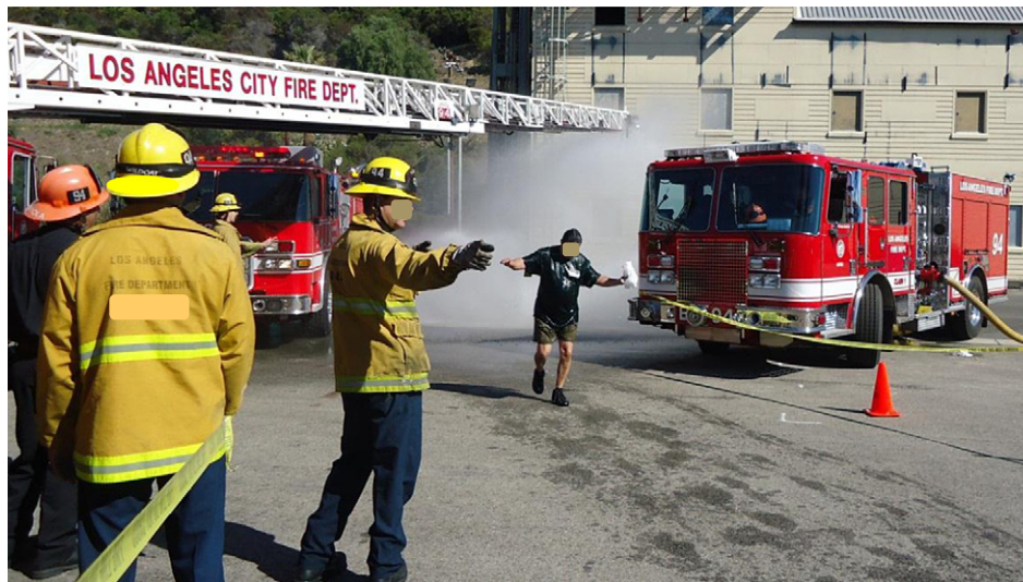
Fig. 6. Demonstration of the ladder pipe system (LPS) for mass casualty decontamination. Individuals are directed to walk through a high volume water mist generated by overhead and side fogging nozzles from two adjacent fire tenders. Reproduced with permission of the US Department of Health and Human Services Biomedical Advanced Research and Development Authority (2013).
