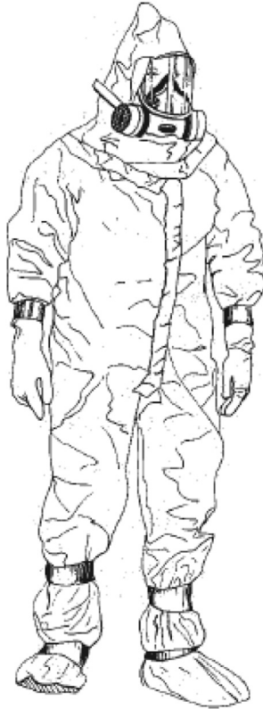
Fig. 3. Level C personal protective equipment. (From ATSDR. Managing Hazardous Material Incidents (MHMI) . Volumes 1, 2, and 3. Agency for Toxic Substances and Disease Registry (ATSDR). Atlanta (GA): U.S. Department of Health and Human Services, Public Health Service; 2001. Available at: http://www.atsdr.cdc.gov/MHMI/index.asp . Accessed July 15, 2014).
