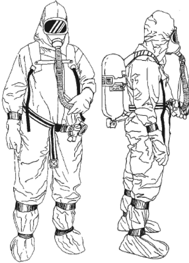
Fig. 2. Level B personal protective equipment. (From ATSDR. Managing Hazardous Material Incidents (MHMI). Volumes 1, 2, and 3. Agency for Toxic Substances and Disease Registry (ATSDR). Atlanta (GA): U.S. Department of Health and Human Services, Public Health Service; 2001. Available at: http://www.atsdr.cdc.gov/MHMI/index.asp . Accessed July 15, 2014).
